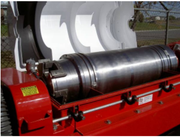
Tec-1655-FVS Centrifuge Solids Discharge End
