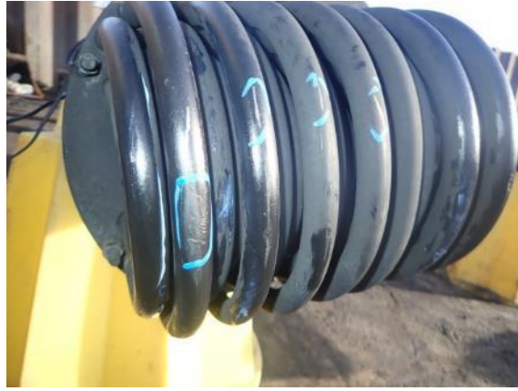
Figure 26. Mechanical damage to bundle from bundle removal;
