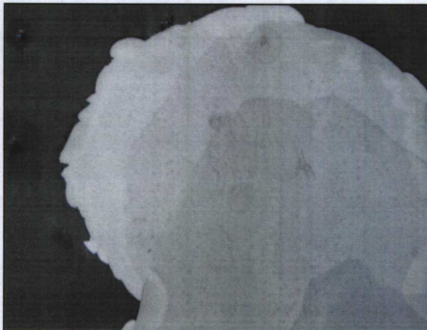
FIGURE 5. VESSEL 3497-2: SHOWS INTACT FIRST COAT BENEATH REMOVED BLISTER. THE AREAS OF DARKENING LIKELY CORRESPOND TO THE INGRESS OF FLUIDS DURING SERVICE EXPOSURE.
