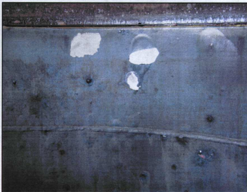
FIGURE 3. VESSEL 3497-2: SHOWS BLISTERS THAT OCCURRED BETWEEN THE FIRST AND SECOND COATS.
