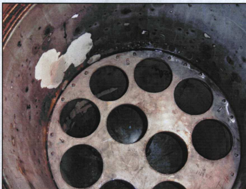
FIGURE 4. VESSEL 3497-2: SHOWS DISCOLORATION DUE TO SERVICE AND THE EXTENT OF THE POOR ADHESION BETWEEN BLISTERED FINISH COAT AND WELL-BONDED FIRST COAT.
