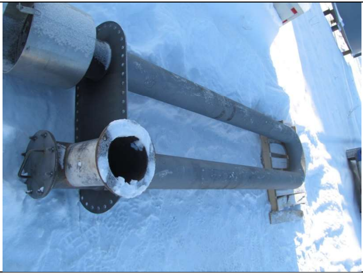
Fire tube after sand blasting
