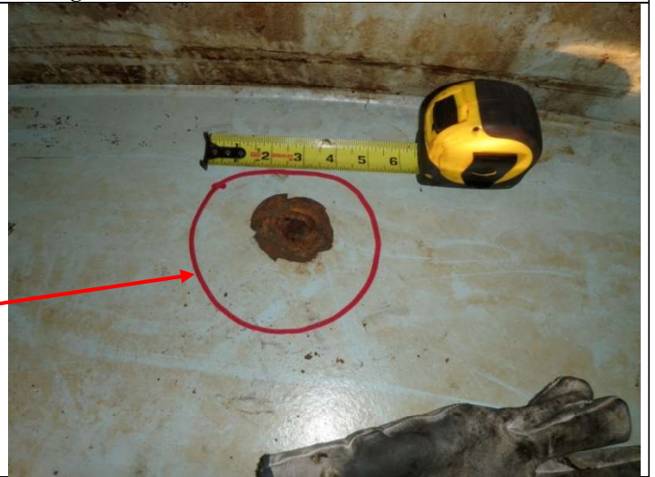
Through hole - 3.0 inches dia.
