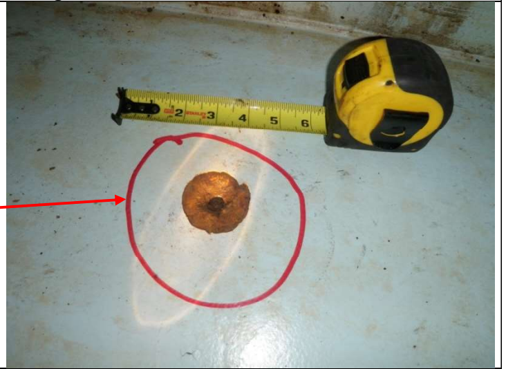
Through hole 2.5 inches dia.
