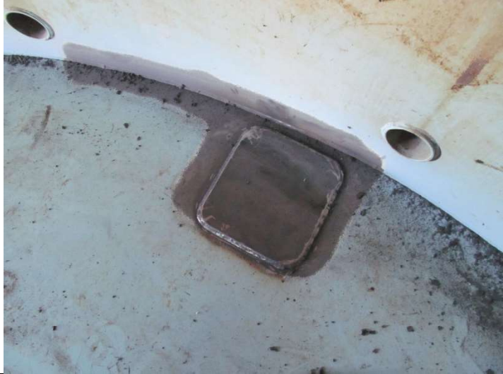
Welded Patch Nov 22
