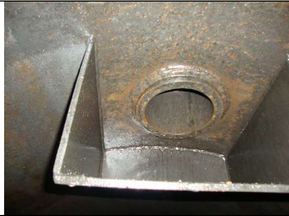
Inlet nozzle and deflector plate
