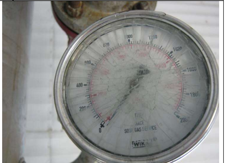
Pressure gauge – Damaged gauge glass
