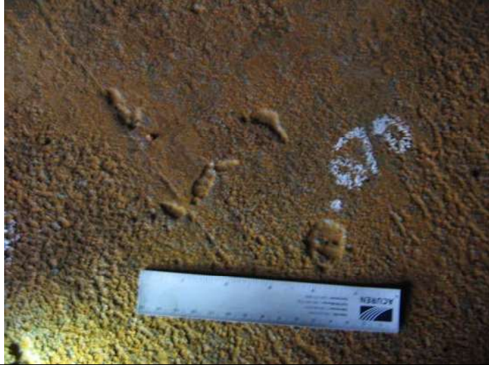
Pits at bottom of shell.
