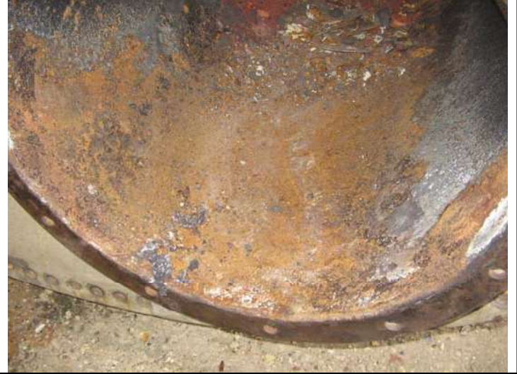
Corrosion along bottom ID of exhaust end of firetube.
