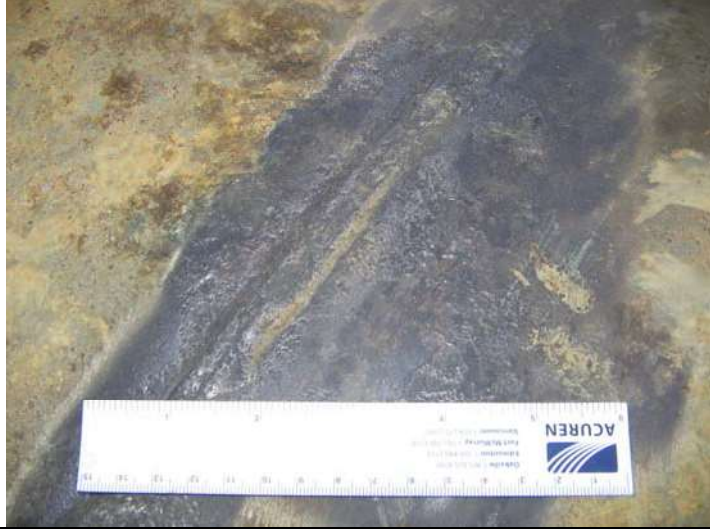
Corrosion along top of firetube.
