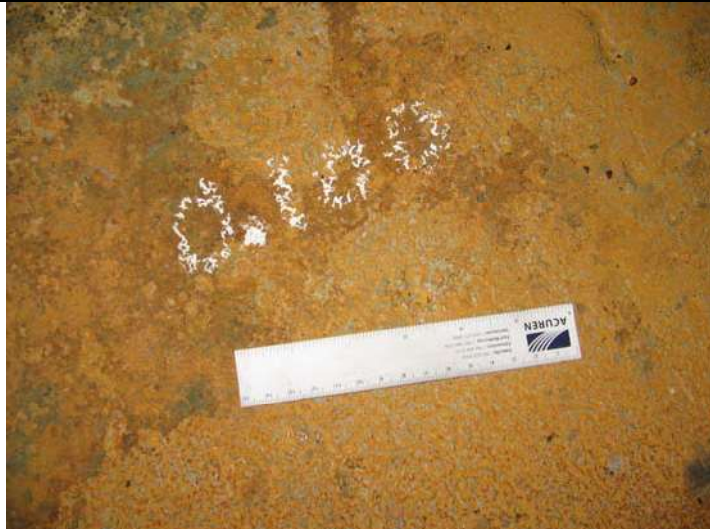
Pitting along the bottom of the shell (glycol side.)
