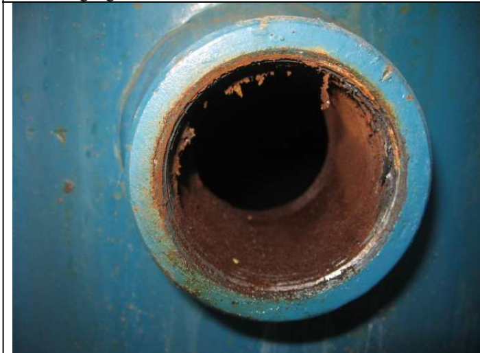
Water dump control opening – general oxidization and surface corrosion – no pitting.
