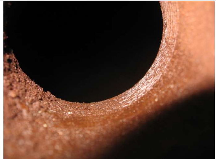
Water dump control nozzle – surface corrosion – no pitting.
