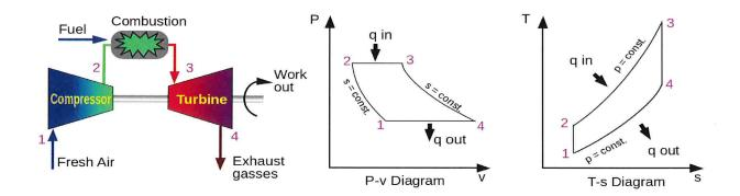
The idealized Brayton cycle where P = pressure, V = volume, T = temperature, S = entropy, and Q = the heat added to or rejected by the system.
