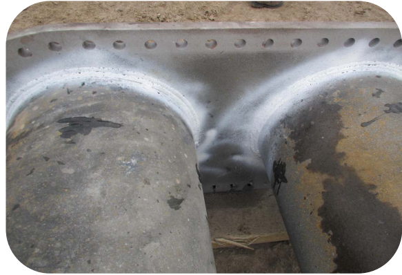
A2710237_Tube to tube sheet MPI_10Oct2012
