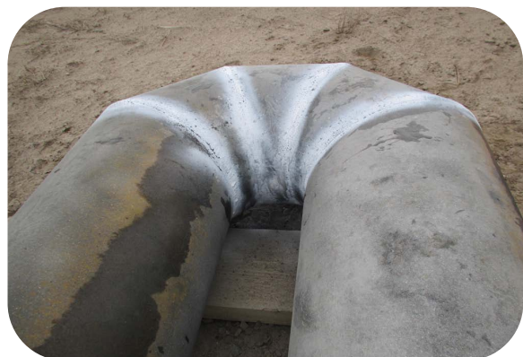
A2710237_MPI of the miter joints_10Oct2012
