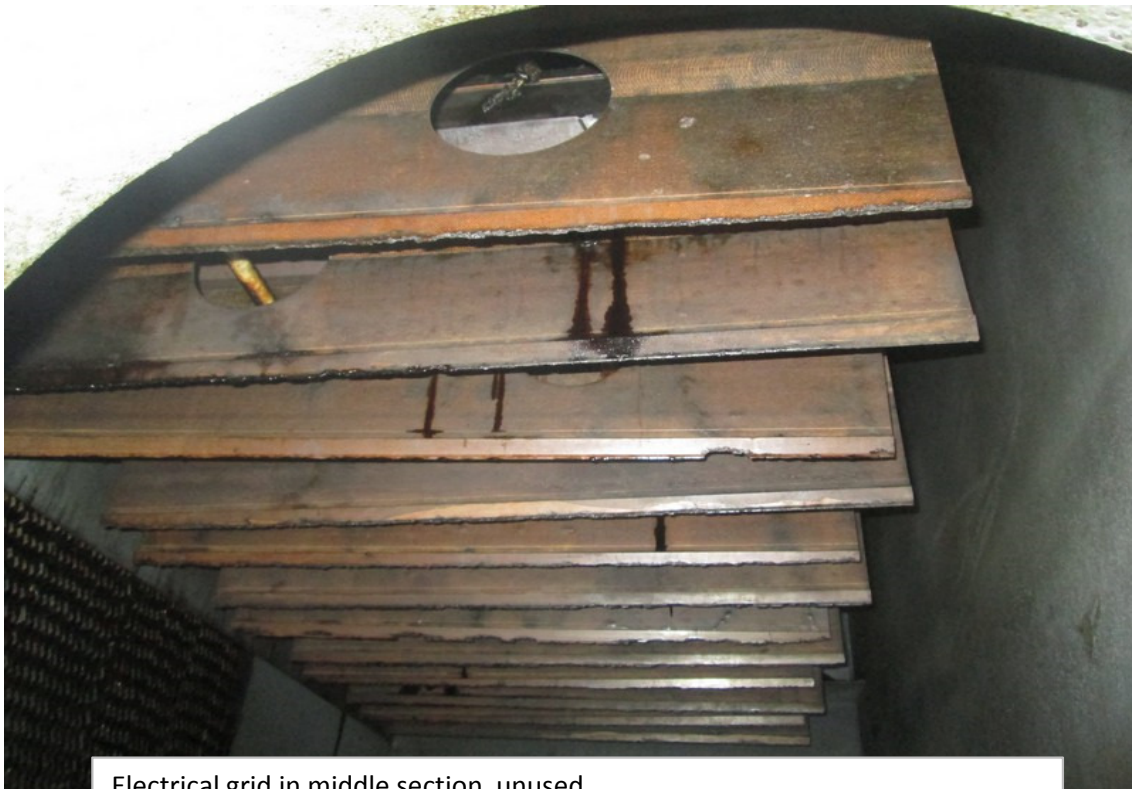
Middle section. Anodes in vessel, 70% remaining. Baffle group intact.
