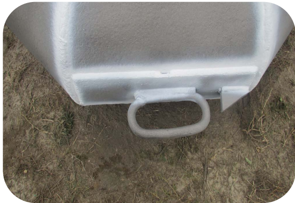
A2710237_MPI of the lifting lug to repad and repad to miter section shell_9Sept2014
