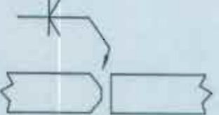
Figure 15 Double Bevel Butt
