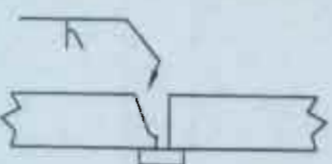
Figure 11 Single J Butt with Backing Strip
