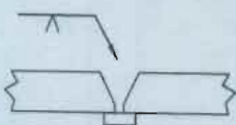
Figure 5 Single Vee Butt with Backing Strip
