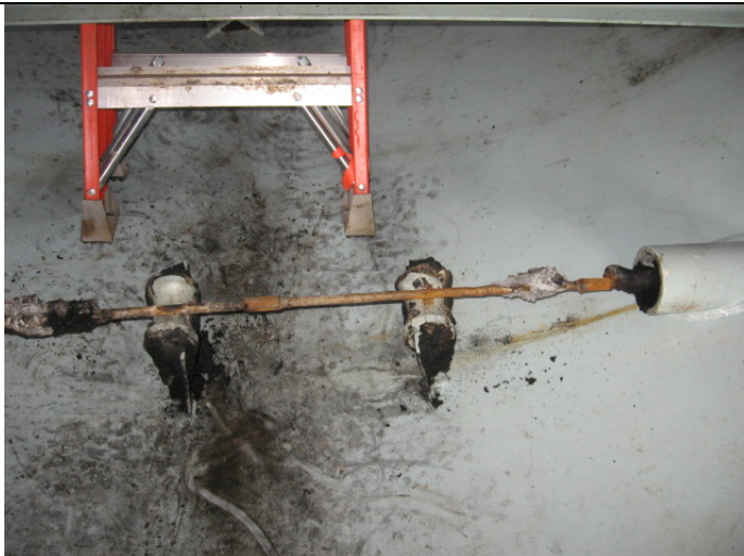
Anode in front end – completely consumed.
