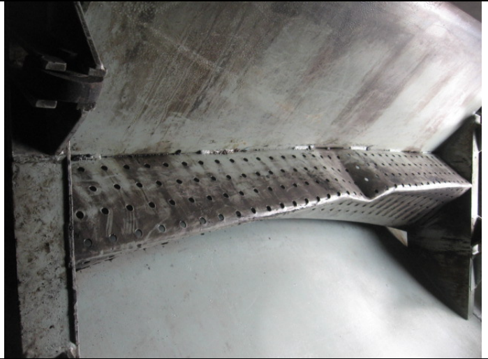
Sparging chutes in front end – severe deflection and distortion.
