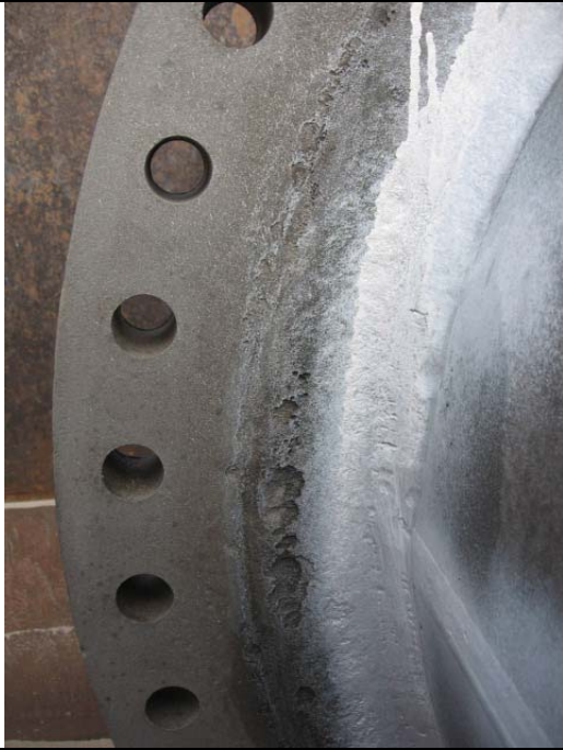
Deep pitting to .220 inches on fire tube flange area outside of gasket seating area.
