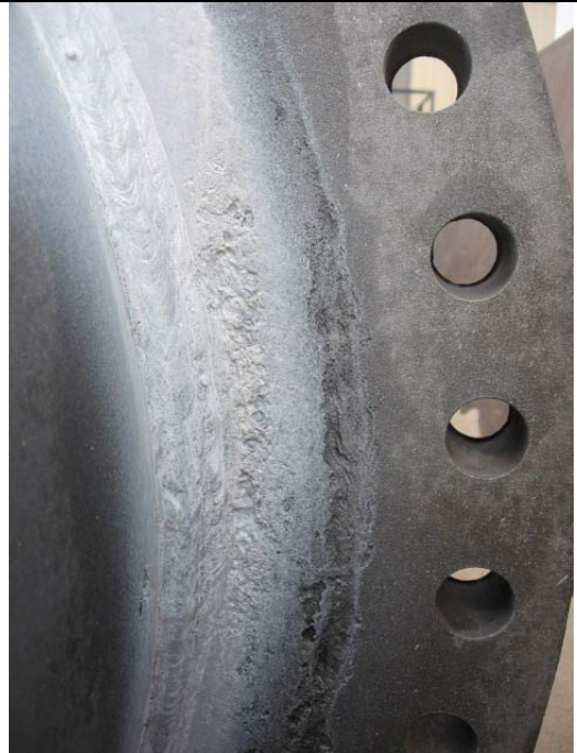
Pitting on internal side of flange but no on gasket seating face to .140 inches deep
