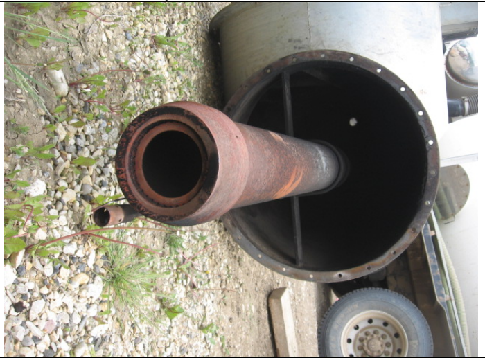
Burner nozzles – free of obstructions
