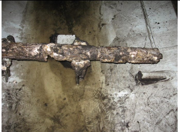
Sparging chutes in front end – severe deflection and distortion.
