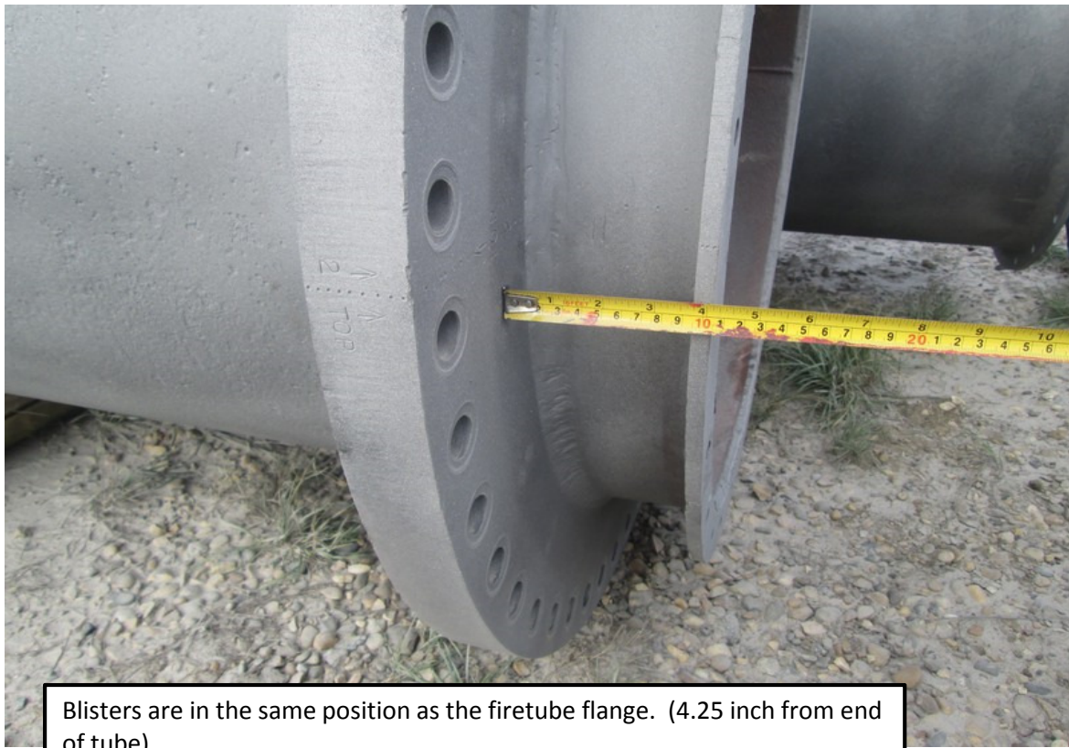
Small blister dimensions. Blister height = 4 mm, steel thickness = 13 mm.
