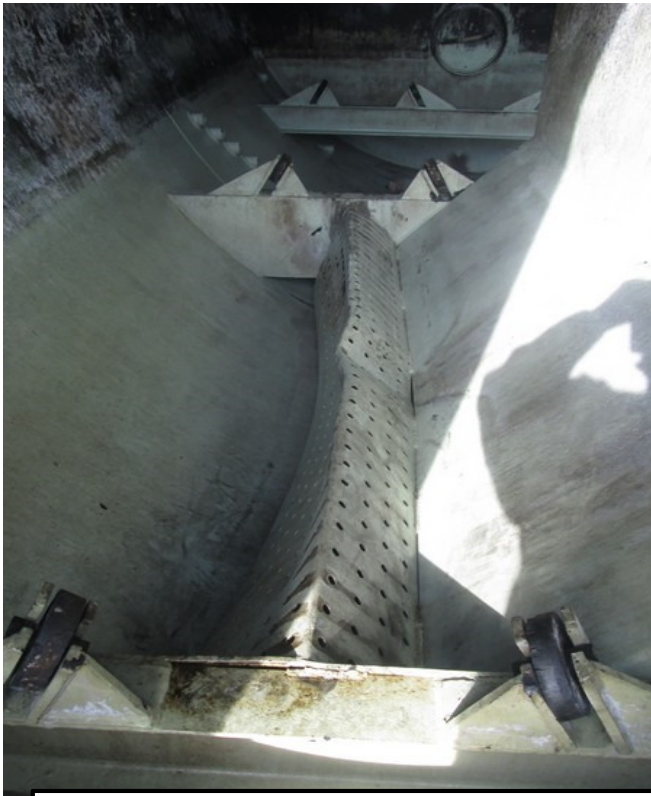
Both left and right shrouds below firetubes are bent. Coating damage is limited to shroud and nozzles/anode holders. No coating damage to pressure boundary.
