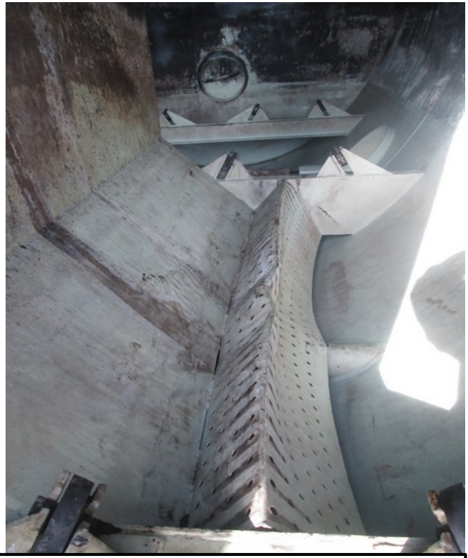
Both left and right shrouds below firetubes are bent. Coating damage is limited to shroud and nozzles/anode holders. No coating damage to pressure boundary.
