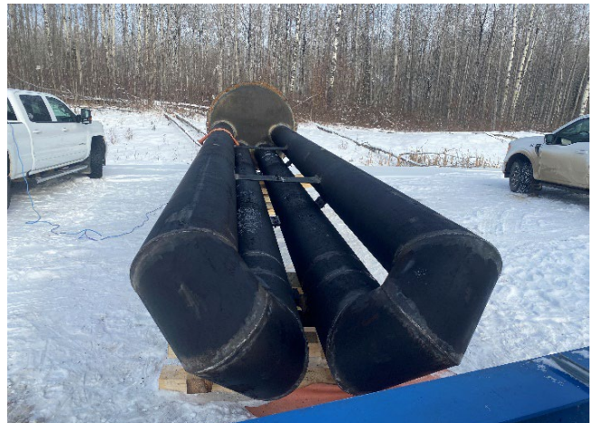
Picture 16 Burner Tubes
