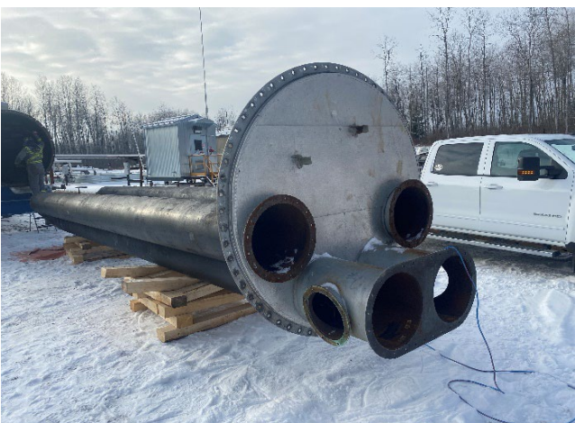
Picture 17: Burner Tube and North End Plate
