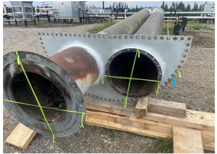
ATMOSPHERE SIDE OF TUBESHEET
