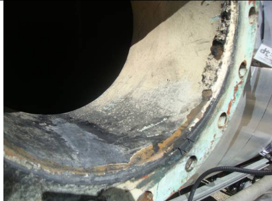
Coating peeling in man way
