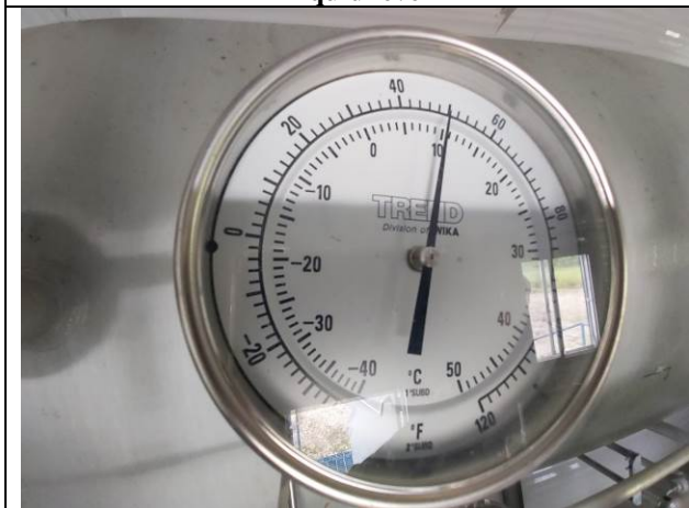
Temperature gauge -40 to 120°F
