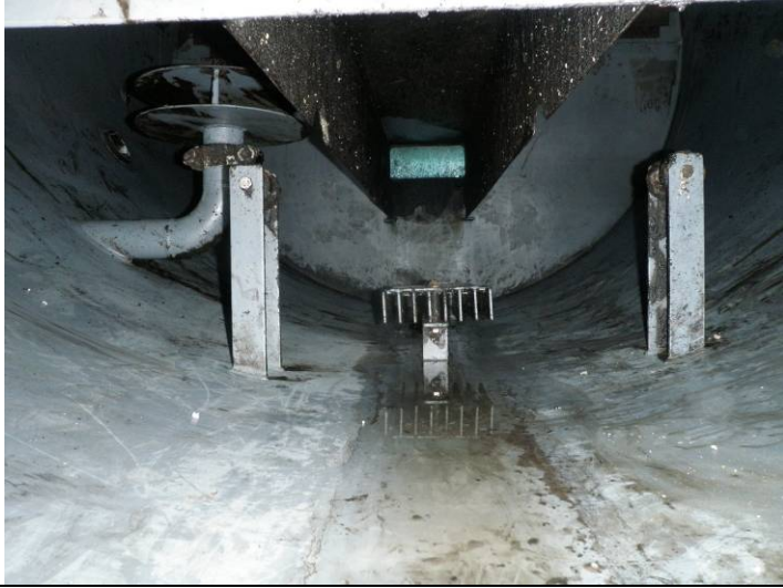
Lower shell/Cathode support/Vortex
