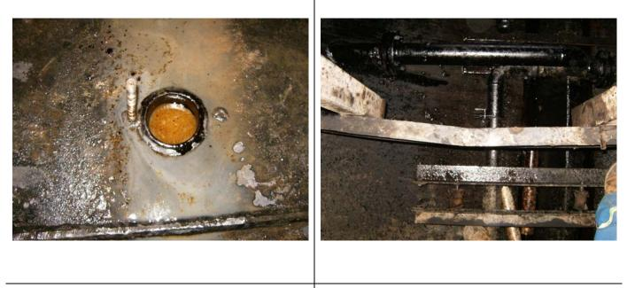
Figure 017\_Broken Anchor Bolt for Vortex Breaker\_22Aug10
