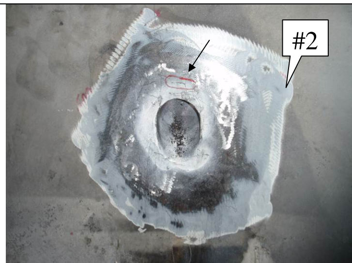
4 inch nozzle – indication detected
