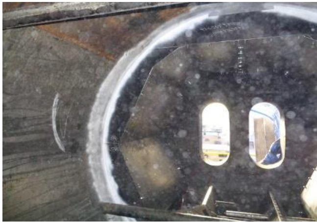
MPI on final inlet horseshoe downcomer to shell fillet welds 12 hours after welding was completed
