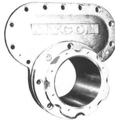
Fig.104 Balance piston cover and unloader cylinder
