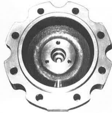
Fig. 39 Body of unloader cover
