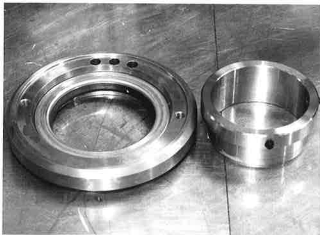
Fig. 146-2 Seal retainer oil seal and sleeve (2003 May~)
