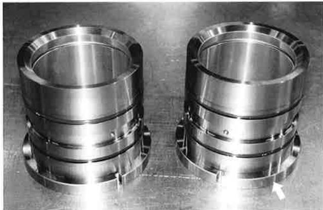
Fig. 85 Notch in bearing
