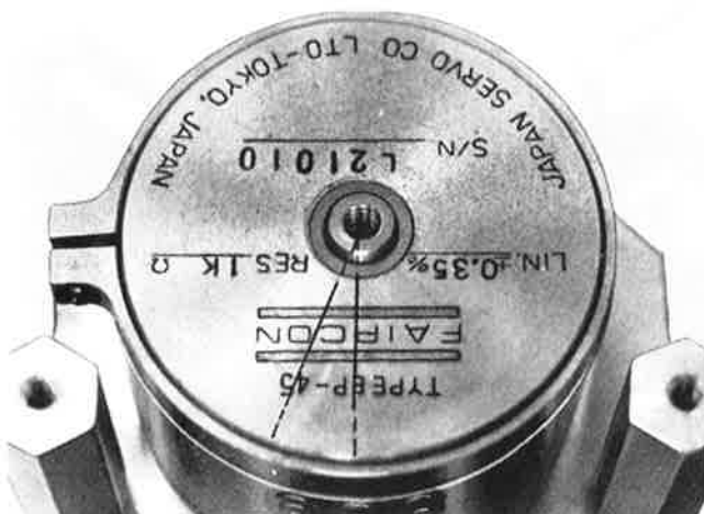
Fig. 162 Adjustment of potentiometer at no-load position
