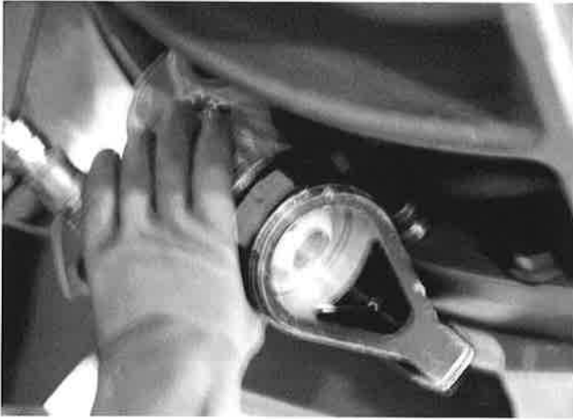
Fig. 102 Fastening of bolts by hydraulic wrench (320-400UD)
