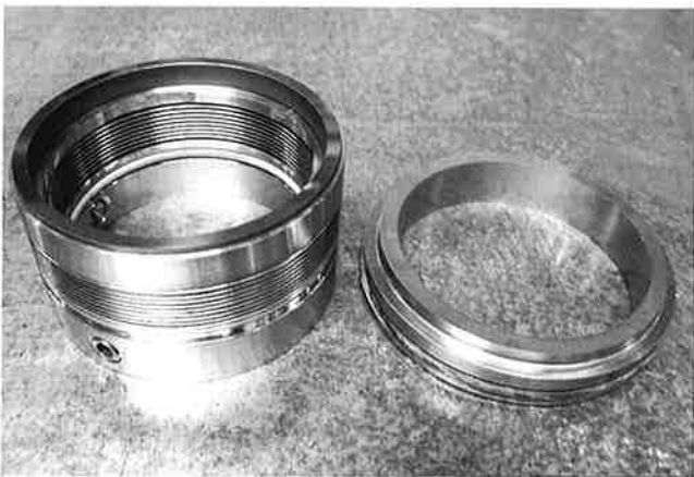
Fig. 29 Bellows type single seal
