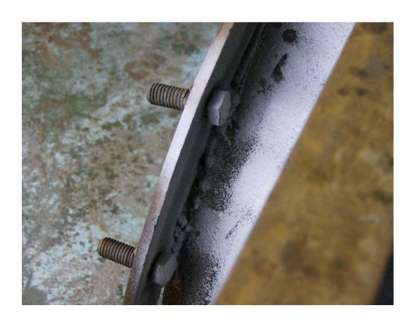
A0161747\_External Fillet Weld-Minimal Fusion&Reinforcement\_06Jun07
