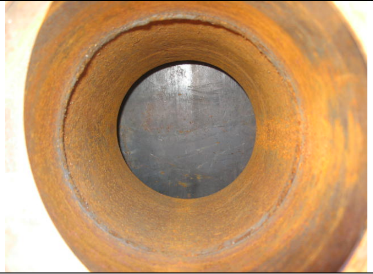
Inlet nozzle showing deflector plate
