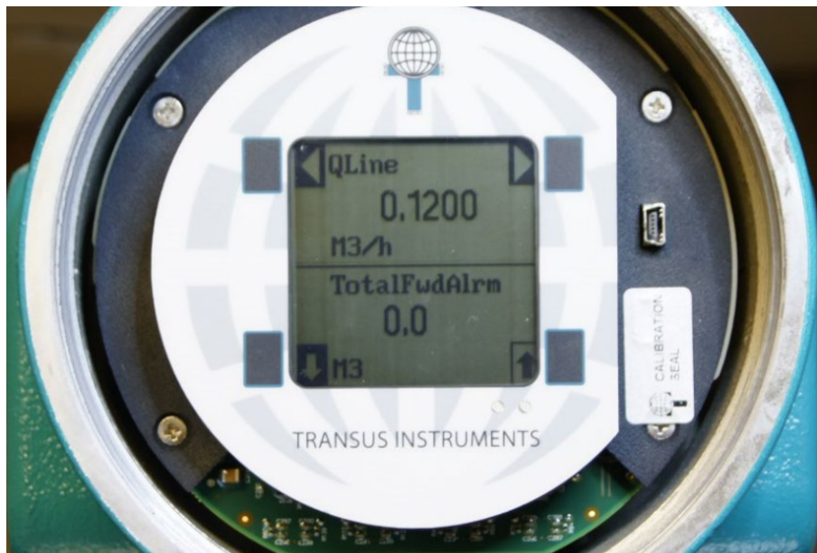
Figure 6-1 - LCD and keypad (front cover removed)
