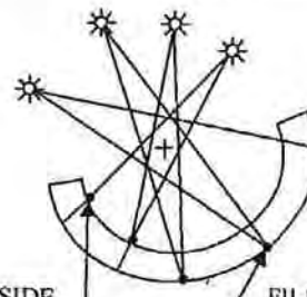
CURVED COMPONENTS WITH RADIATION SOURCE TO FILM DISTANCE GREATER THAN RADIUS OF CURVATURE.
